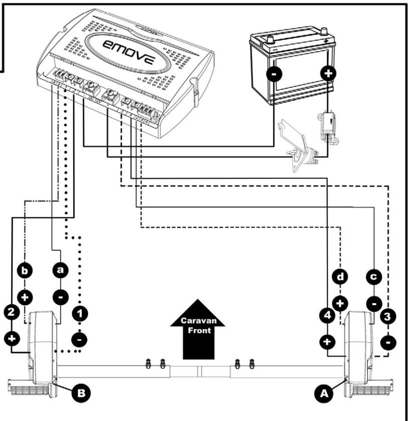
Parts Identification & Fitting Diagrams
